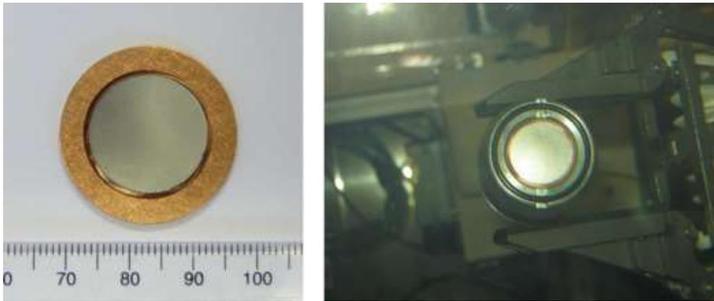
Figure 5: (top left) TRIUMF-designed, GE PETtrace solid target capsule; (top right) (Schaffer, 2014) (SK Zeisler, 2014) with mounted  $^{100}\text{Mo}$  target (bottom left) enriched  $^{100}\text{Mo}$  target mounted on a copper test backing; (bottom right) enriched  $^{100}\text{Mo}$  after 6hr, 130  $\mu\text{A}$  irradiation (Schaffer, 2014)
